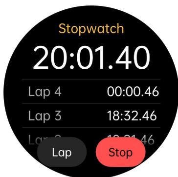
1. Press the rotating crown to enter the application center, and click "Stopwatch" to enter the stopwatch interface.
