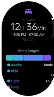
Wear the watch to sleep, and it will automatically recognize when you enter sleep, wake-up times, as well as durations of deep sleep, light sleep, rapid eye movement, and wakefulness.
