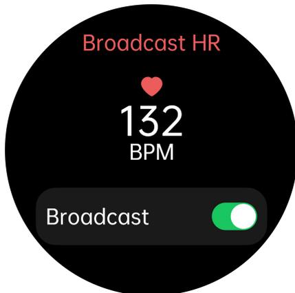
Turning on heart rate broadcasting can push the watch's heart rate to devices that support external standard Bluetooth heart rate.
